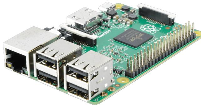
Figura 2.11: Modelo Raspberry Pi 2 B.
