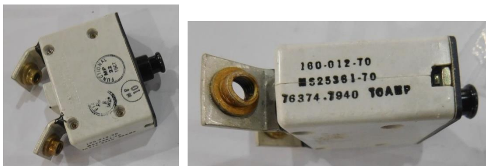
Figura 7: Disyuntor P/N MS25361-70
