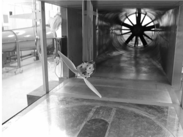
Figure 1. Photograph of test section with experimental rig installed.
