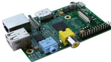
Ilustración 34: Raspberry Pi Model B [Fuente: [www.raspberrypi.org](http://www.raspberrypi.org)]
