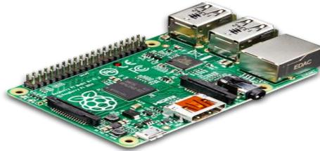
Ilustración 33: Raspberry Pi 2 Model B [Fuente: [www.raspberrypi.org](http://www.raspberrypi.org)]
